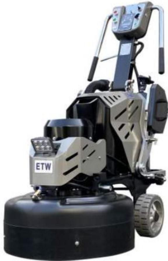
My understanding is that a walk behind concrete grinder was used to grind the UHPC. UHPC is formed and poured  $\frac{1}{4}$ " high. The reason we overpour  $\frac{1}{4}$ " is to expose air pockets and other anomalies occurring during placement. Grinding removes these imperfections leaving a smooth surface.
