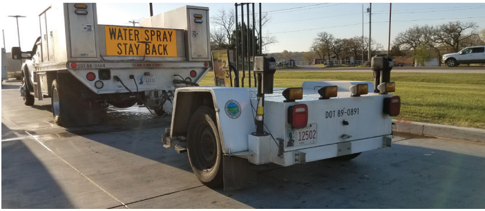
Left: ODOT Skid Tester; Above: OSU GripTester. Photos courtesy Josh Li.
