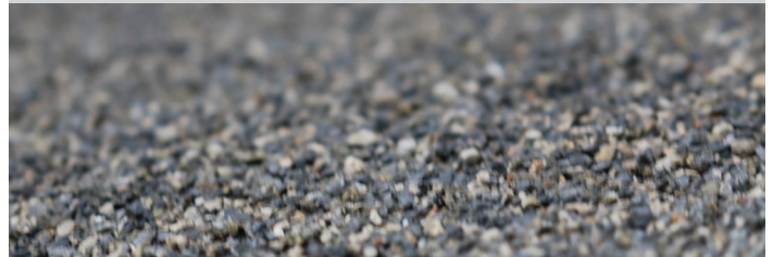
High Friction Surface Treatment has a coarse finish of rough-edged aggregate.
