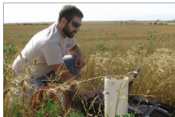
Water-level data from hourly recorders help determine periodic influences on the aquifer.
