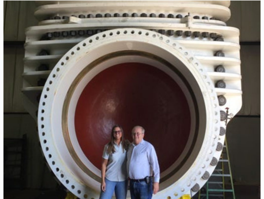
Resident engineer Shelly Hatton and Jack Stevens, TRWD board president, stand in front of the four-story custom-built gate valve that became part of the North Texas Integrated Pipeline Project. Photo courtesy TRWD
