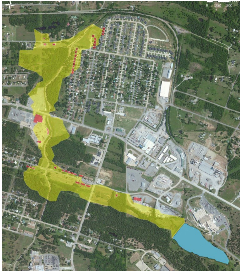
Figure 1. Breach inundation map
