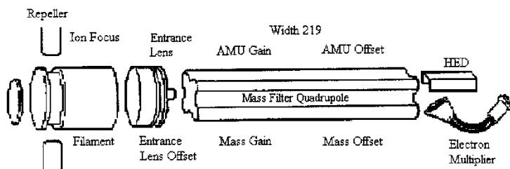
of Rf and DC voltage values, only ions of a specific mass to charge ( $m/z$ ) will traverse the length of the open space between the rods. All other ions are neutralized as they strike the surface of the rods. During a typical run, the MS scans
