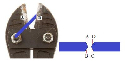
If the working surface of the tool is larger than the test medium, ensure the test toolmarks are labeled to represent which area they were made with.
