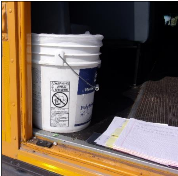
Bus 62 – Unsecured Trash Can Blocking Exit Door
