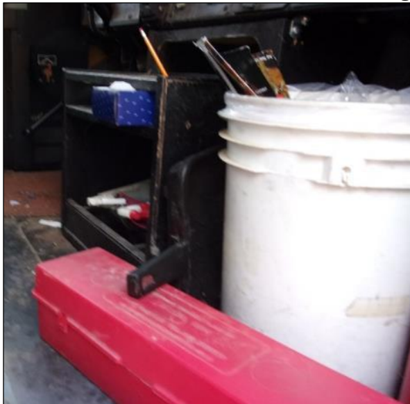
Bus 13 – Unsecured Trashcan Overflowing
