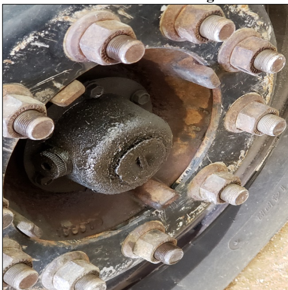
Wheel Seal Leaking
