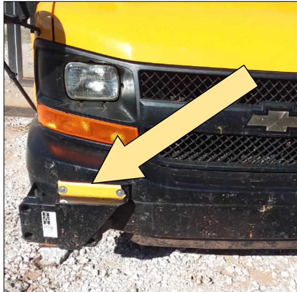
Broken Crossing Arm
