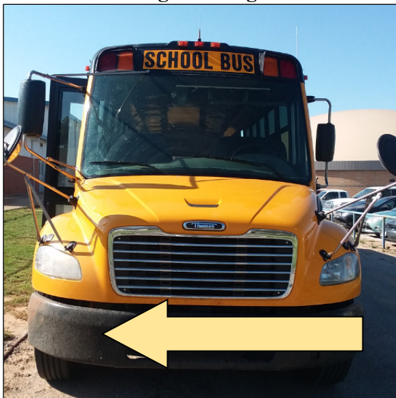
Missing Crossing Arm
