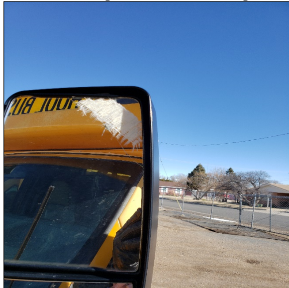
Mirror Repaired with Duct Tape
