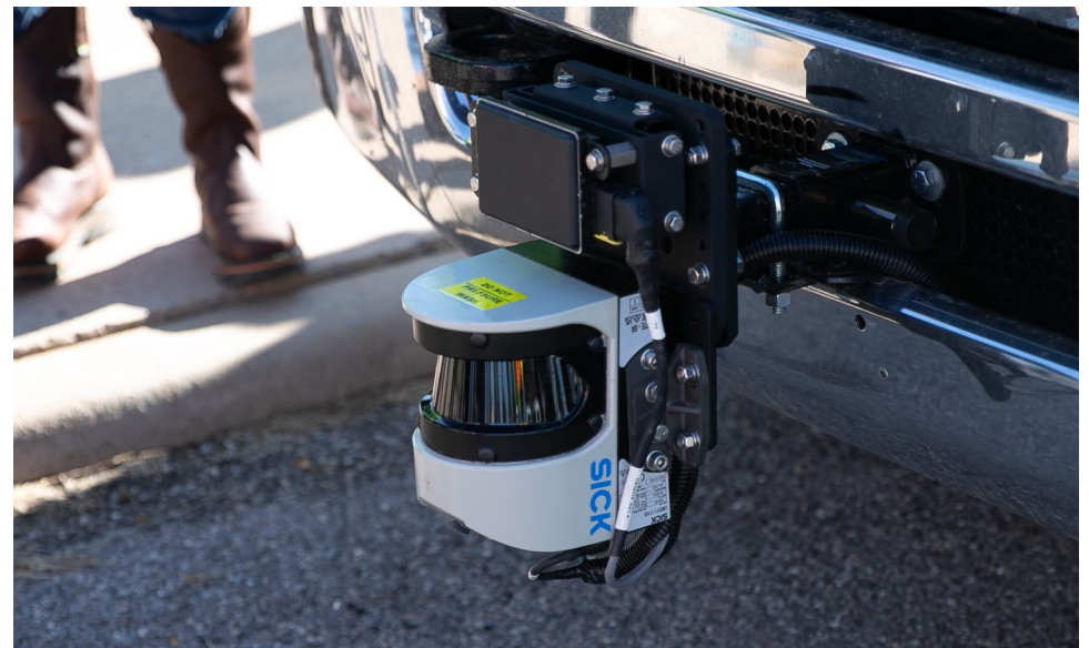
This ATMA LiDAR device detects obstacles and monitors the surrounding environment to help prevent collisions. Source: ODOT
