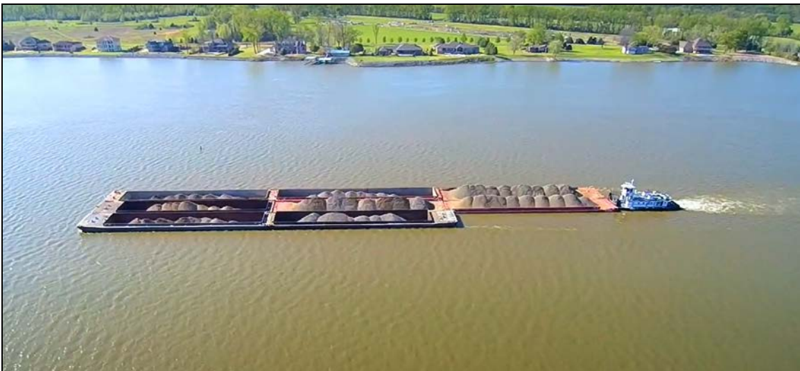
Figure 5.2-2: Typical Hopper Barge Tow in Transit
