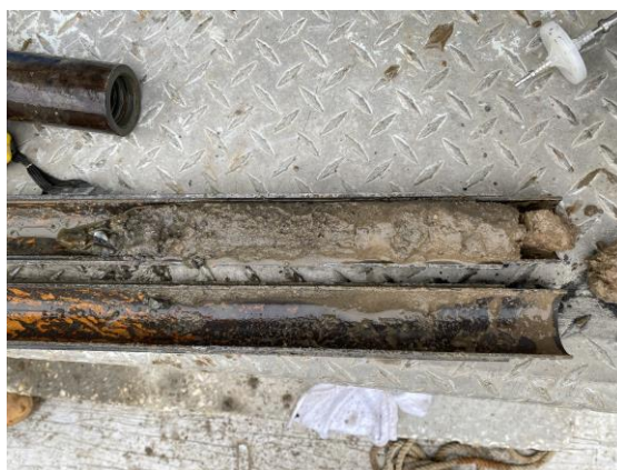
Photo #6: Representative photo of SB-10 (2-4 ft below mudline).
