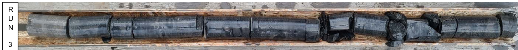
Photo # 3 Run 3 of boring B-2 was from 44 to 49 feet. Run 3 had a recovery of 87% and an RQD of 8%.
