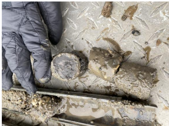
Photo #7: Representative photo of SB-10 top of bedrock.
