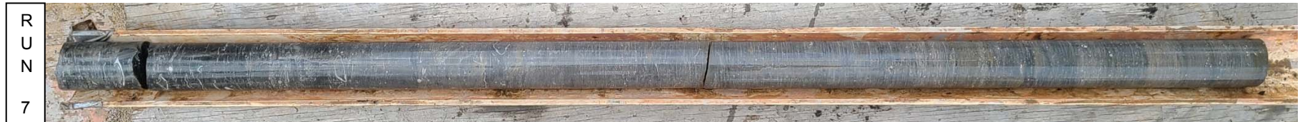
Photo # 7 Run 1 of boring B-6 was from 42 to 47 feet. Run 2 had a recovery of 100% and an RQD of 95%.
