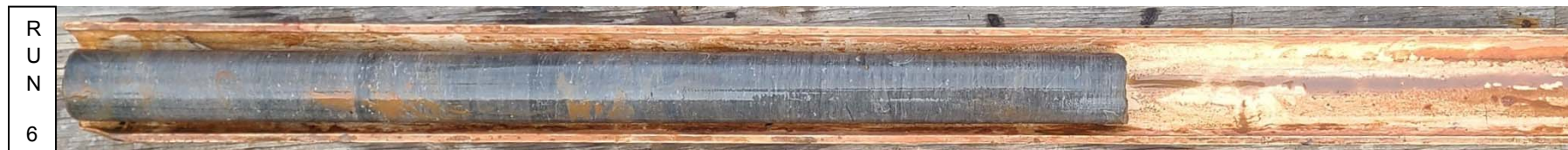
Photo # 6 Run 1 of boring B-6 was from 39.5 to 42 feet. Run 1 had a recovery of 100% and an RQD of 100%.
