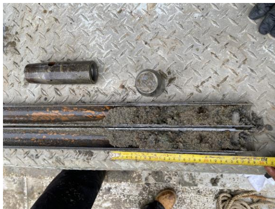
Photo #10: Representative photo of SB-11 top of bedrock.
