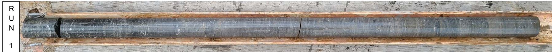
Photo # 1 Run 1 of boring B-2 was from 34 to 39 feet. Run 1 had a recovery of 90% and an RQD of 90%.
