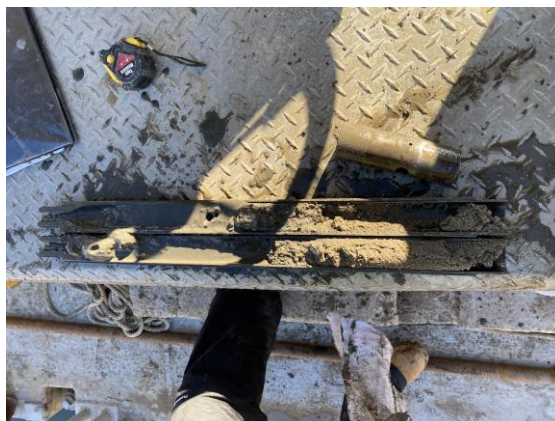
Photo #12: Representative photo of SB-12 (6-8 ft below mudline).
