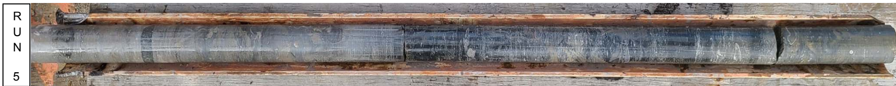
Photo # 5 Run 2 of boring B-4 was from 41.7 to 46.7 feet. Run 2 had a recovery of 100% and an RQD of 100%.
