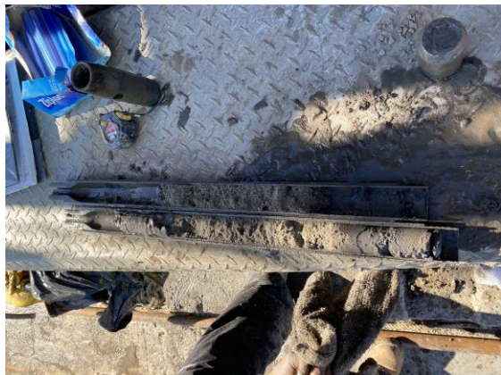
Photo #19: Representative photo of SB-14 top of bedrock.
