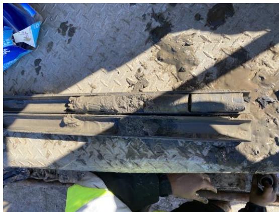
Photo #16: Representative photo of SB-13 top of bedrock.
