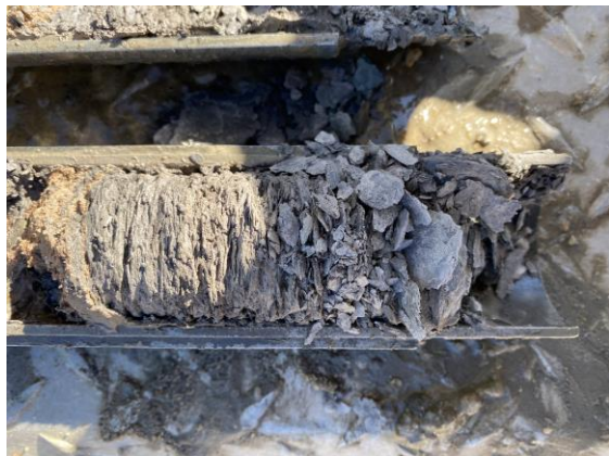
Photo #13: Representative photo of SB-12 top of bedrock.
