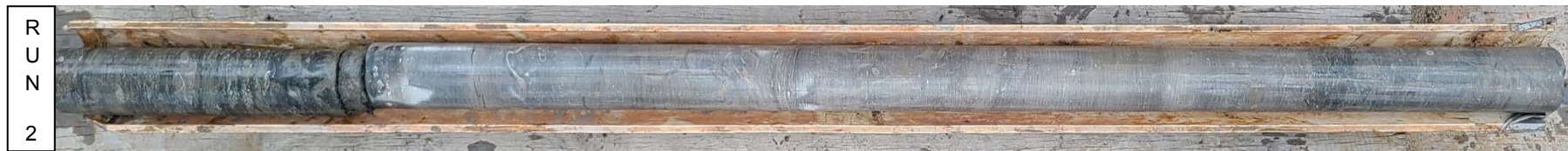
Photo # 2 Run 2 of boring B-2 was from 39 to 44 feet. Run 2 had a recovery of 100% and an RQD of 100%.
