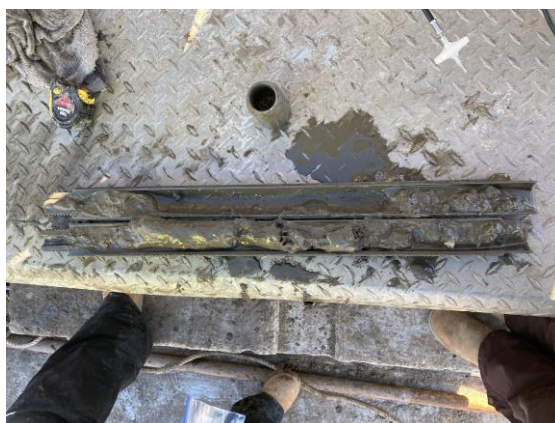
Photo #24: Representative photo of SB-16 (6-8 ft below mudline).
