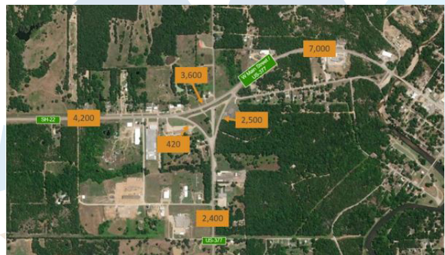
Figure 3: 2022 AADT around project intersection
