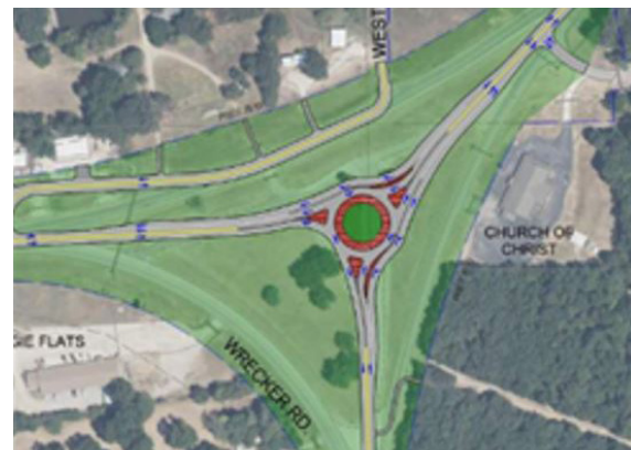
Alternative 3: The Modern Roundabout
