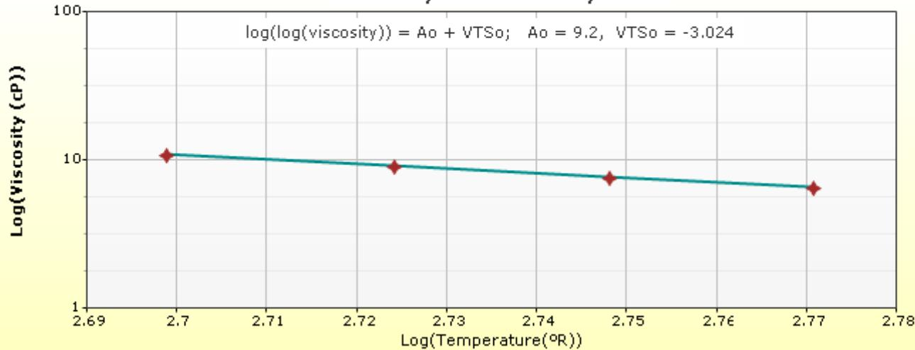
**HMA Layer 2: Layer 2 Flexible : Default asphalt concrete**
