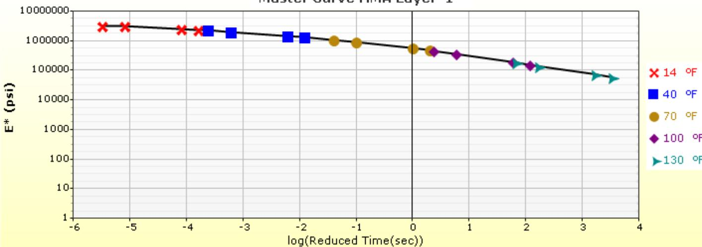
**Shift Curve HMA Layer 1**
