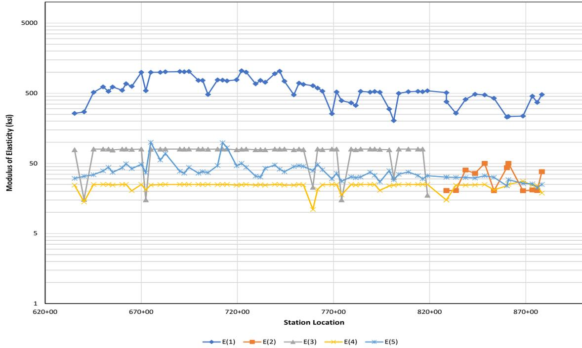
Figure 4 – NB lane back-calculated modulus versus station locations
