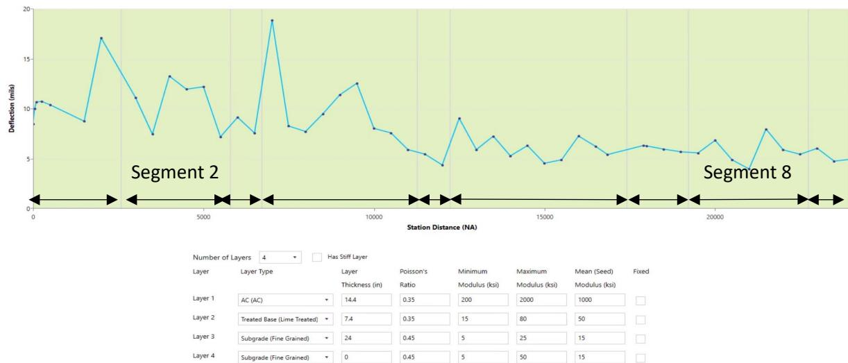
**Figure 3 – SB lane pavement segments, input layer modulus and Poisson's ratio values for back-calculation**
