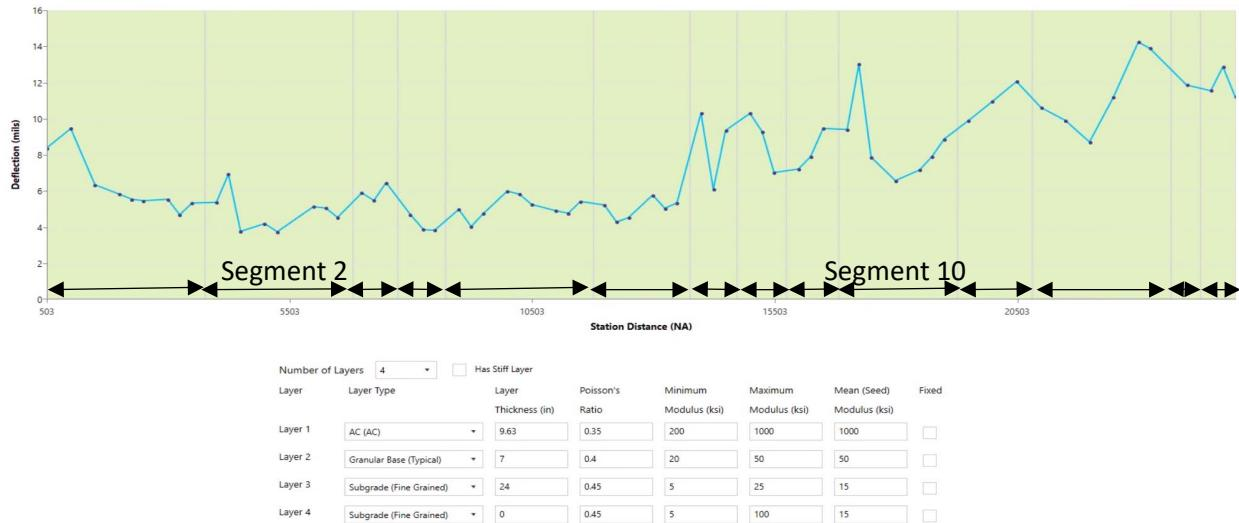
**Figure 2 – NB lane pavement segments, input layer modulus and Poisson's ratio values for back-calculation**
