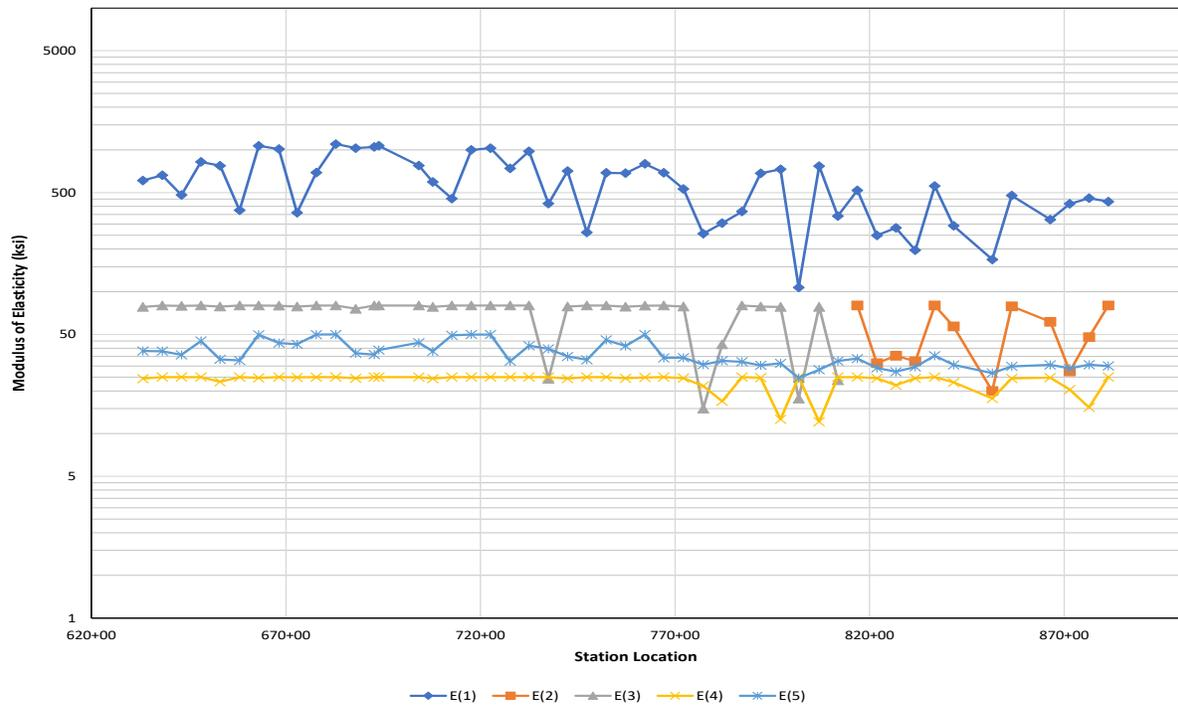
Figure 5 – SB lane back-calculated modulus versus station locations
