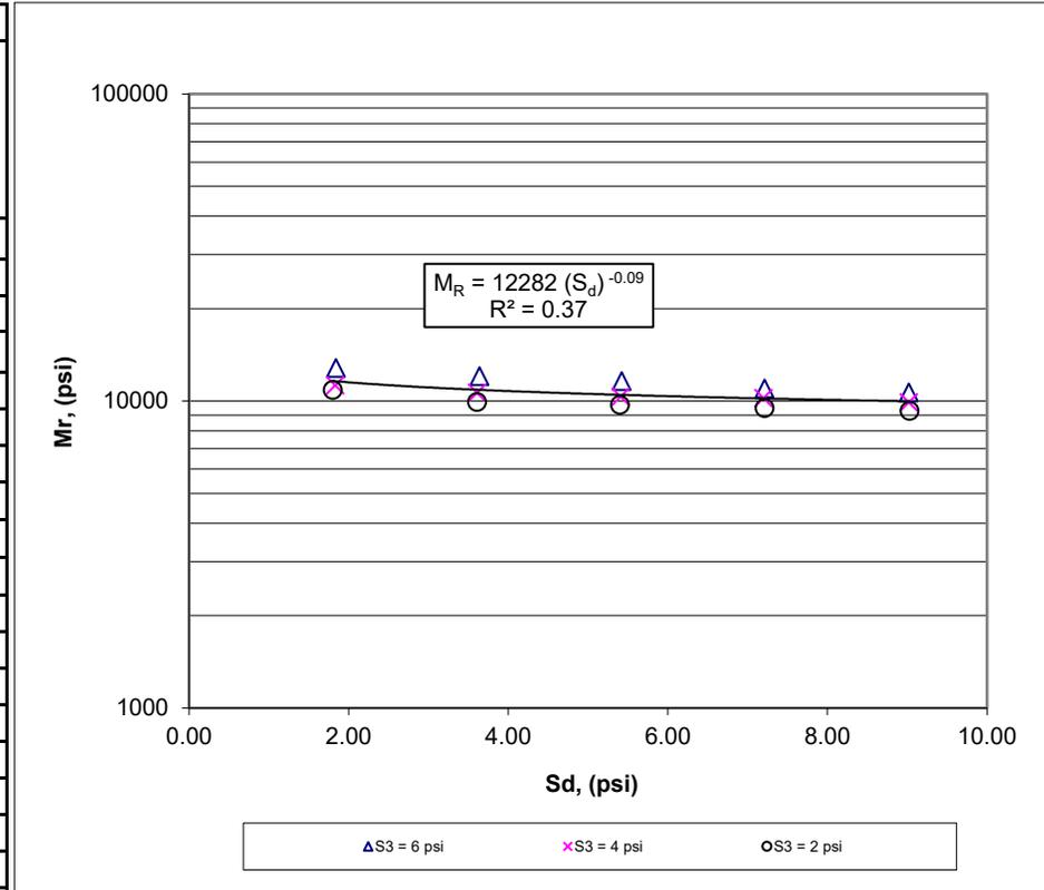
\*Predicted Mr values at the desired applied cyclic stresses using Model #1
