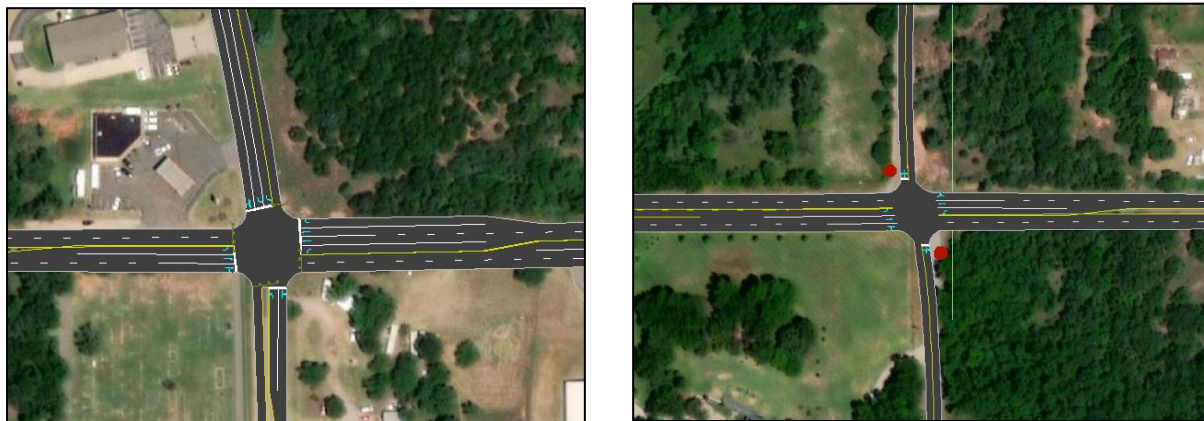
“Ultimate” Configuration Provides Additional Through Lane on Waterloo Road at Sooner Road and Air Depot Blvd. Intersections
