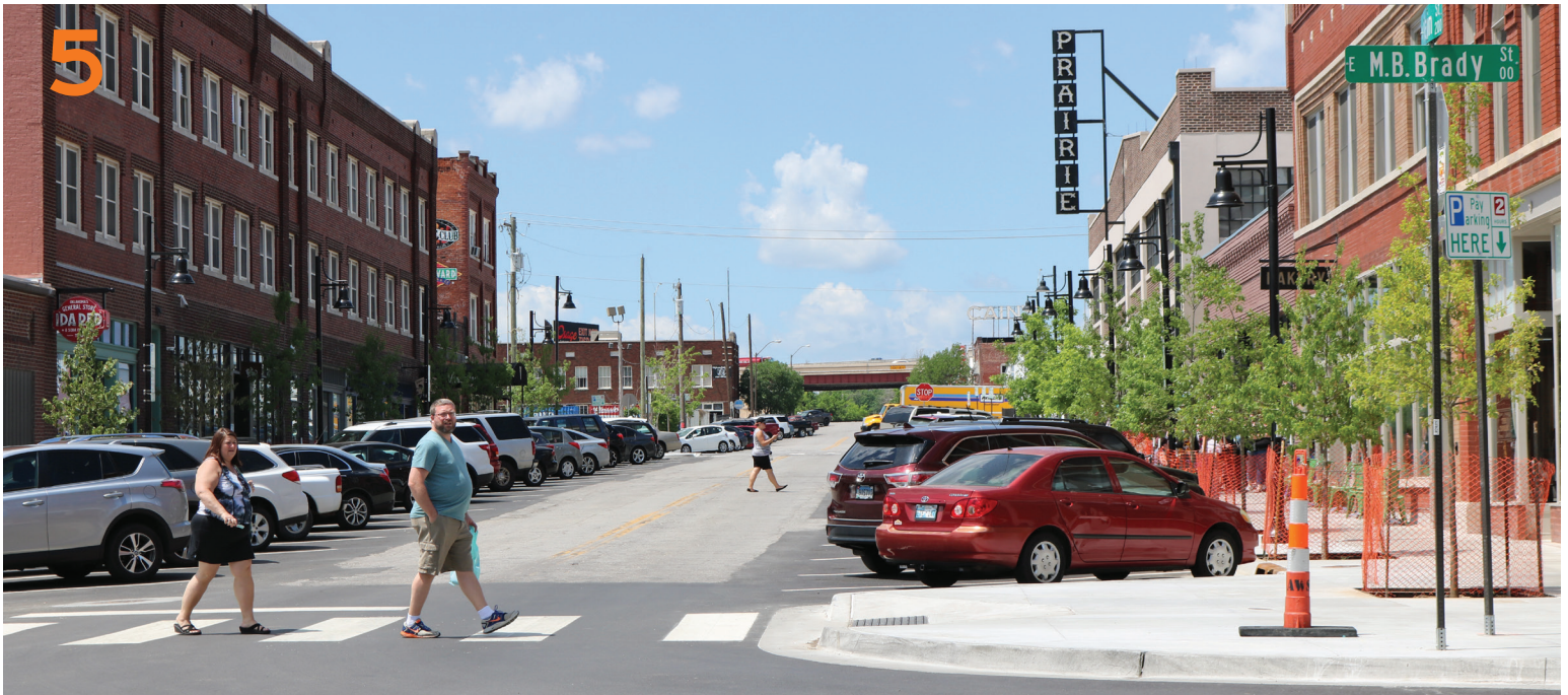
Above: The City of Tulsa reduced the street to two lanes in a road diet within the Brady Arts District, re-using the space to create angled parking and curb extensions that shorten the distance for pedestrians to cross.
