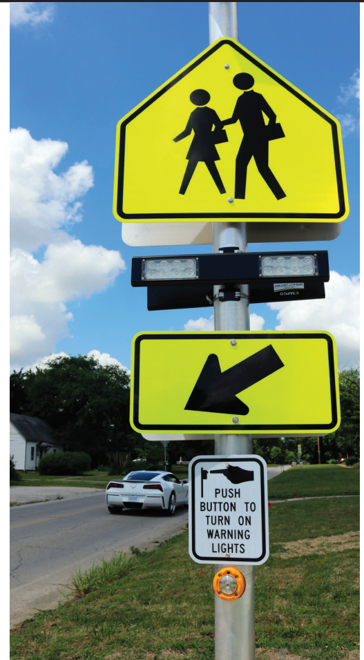
Right: Effective placement and design of pedestrian-activated crossing systems like this solar-powered RRFB in Collinsville, Okla. are outlined by FHWA in the Guide for Improving Pedestrian Safety at Uncontrolled Crossing Locations.
