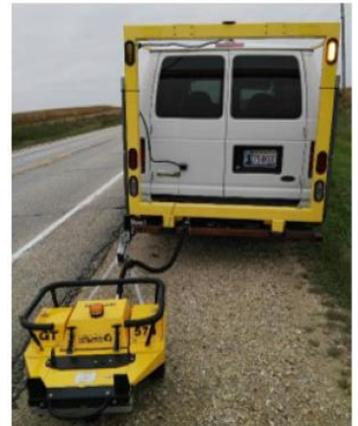
Working closely with ODOT, asphalt and concrete testing sections with various surface characteristics (texture and materials) were selected in Oklahoma as the testing bed for the implementation of Grip Tester. Various operational characteristics of a GT were integrated into the field data collection to evaluate the CFME friction measurements. The data collected at the sites along with
