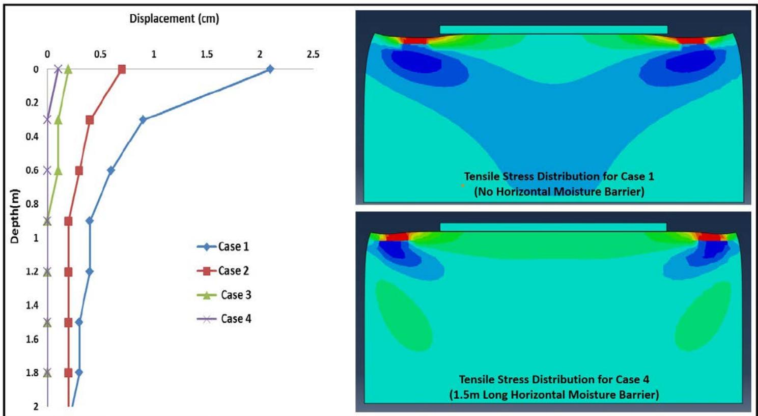
Figure 2 Displacement Profiles for Different Lengths of Moisture Barriers Investigated in this Study
