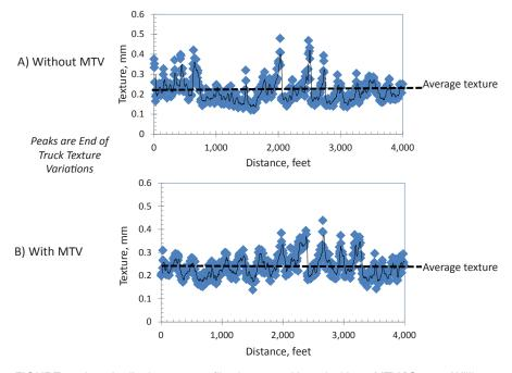
FIGURE 13 Longitudinal texture profile changes with and without MTV [*Source*: Williams (2003)].
