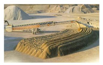
FIGURE 31 Telescoping, radial stacker used to build large scale stockpiles [*Source*: Sam Johnson, Vulcan Materials (n.d.)].
