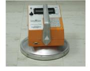
PQI uses measurements of dielectric constant to estimate density.
