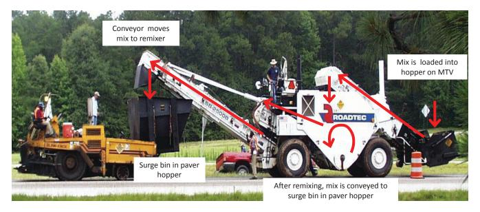
FIGURE 55 Example of remixer as a separate unit [Source: Stroup-Gardiner (2014)].
