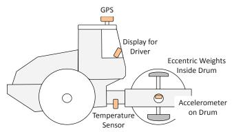
FIGURE 25 Schematic of sensors and electronics used for intelligent compactors [*Source*: Stroup-Gardiner after Haskell (2007); FHWA (2011)].
