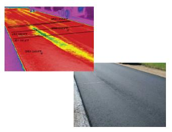
FIGURE 22 Temperature differences that reflect visible changes in texture (longitudinal one-sided segregation) [*Source*: Adams et al. (2001)].
