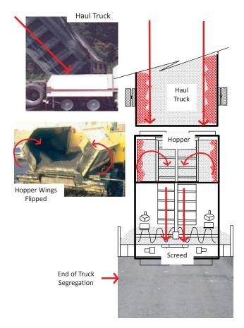
FIGURE 57 End-of-truck segregation: How segregated mix moves from the outer edges of the truck bed to the pavement [*Source*: Stroup-Gardiner (2014)].
