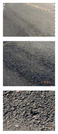
FIGURE 11 Example of severe segregation [*Source*: Gavin and Heath (2002)].
