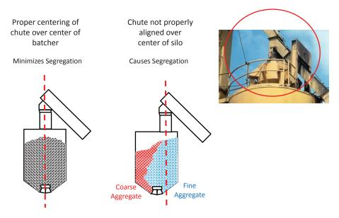
FIGURE 43 Proper use of bin charging batcher over silo [*Source*: Stroup-Gardiner after Murphy (2012a)].
