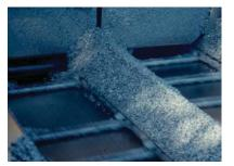
Conventional drag slat configuration can fracture aggregate which shows up behind the screed as a coarser texture.
