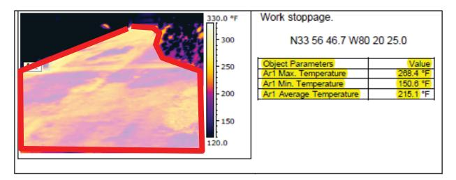
FIGURE 15 Example of standardizing thermal image for analysis by eliminating non-paving areas from the analysis [*Source*: Gunter (2012)].
