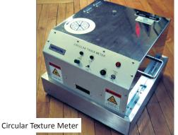
FIGURE 12 Examples of static circular area texture measurement methods [*Source*: Hanson and Prowell (2004); APT (2008)].
