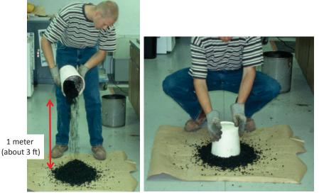
Material inside the bucket diameter is tested and compared to the results for the material outside of the bucket diameter
