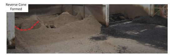
FIGURE 36 Reverse "cone" formed in center of cold feed bin which has been run too low [*Source*: Stroup-Gardiner (2014)].
