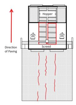
FIGURE 65 Overlay of paver conveyor slat location and the occurrence of longitudinal cracking in the center of lane and on either side of the centerline [*Source*: Stroup-Gardiner after Harmelink et al. (2008)].
