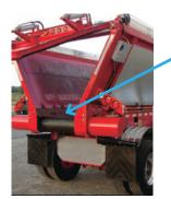
A conveyor belt in the bottom of the truck bed to move the mix out of the back of the truck.
