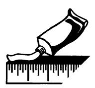
You must check for water in the bottom of the tank at least once each month by smearing a water-finding paste along the bottom of the gauge stick. The paste changes color when it comes in contact with water. Many operators improve their stick readings by smearing a fuel-finding paste on about 6 inches of the stick where they expect the fuel level to be. Fuel-finding paste changes color when it comes in contact with fuel.
