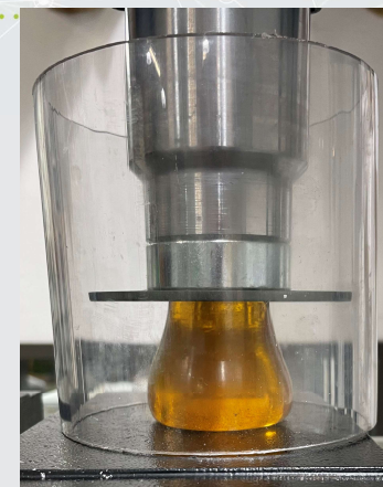
10,000# press test on 1.44" dia. cylinder
