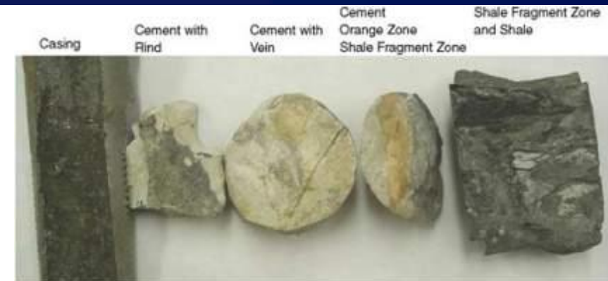
Source: Carey, J.W. et al. Cement with 30 years of CO 2 exposure. Int. J. GHG Control 1 (2007)
