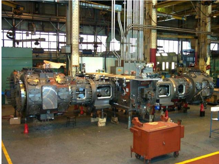
Shop construction of a 5000 hp, 30 MMSCFD compressor
