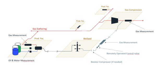
Figure 1 - Closed Loop Gas Capture Schematic
