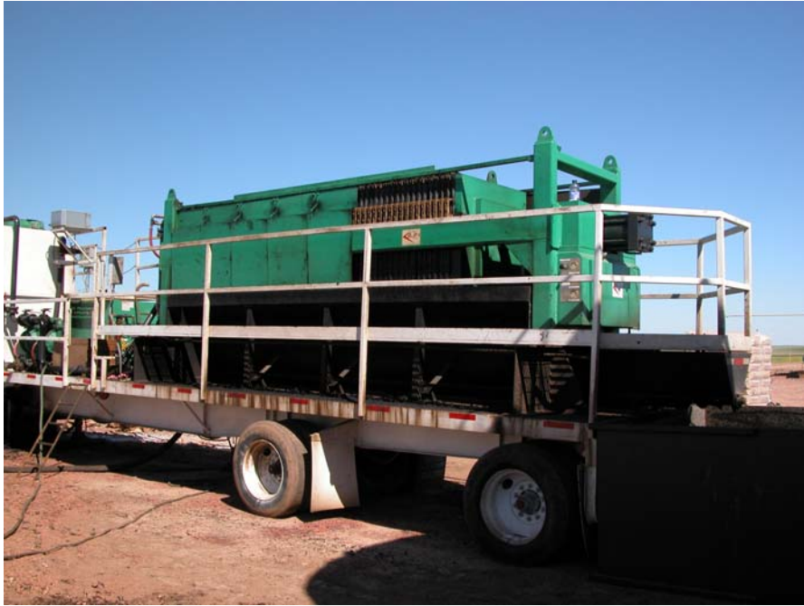
VIEW OF A MOBILE OIL RECOVERY UNIT
