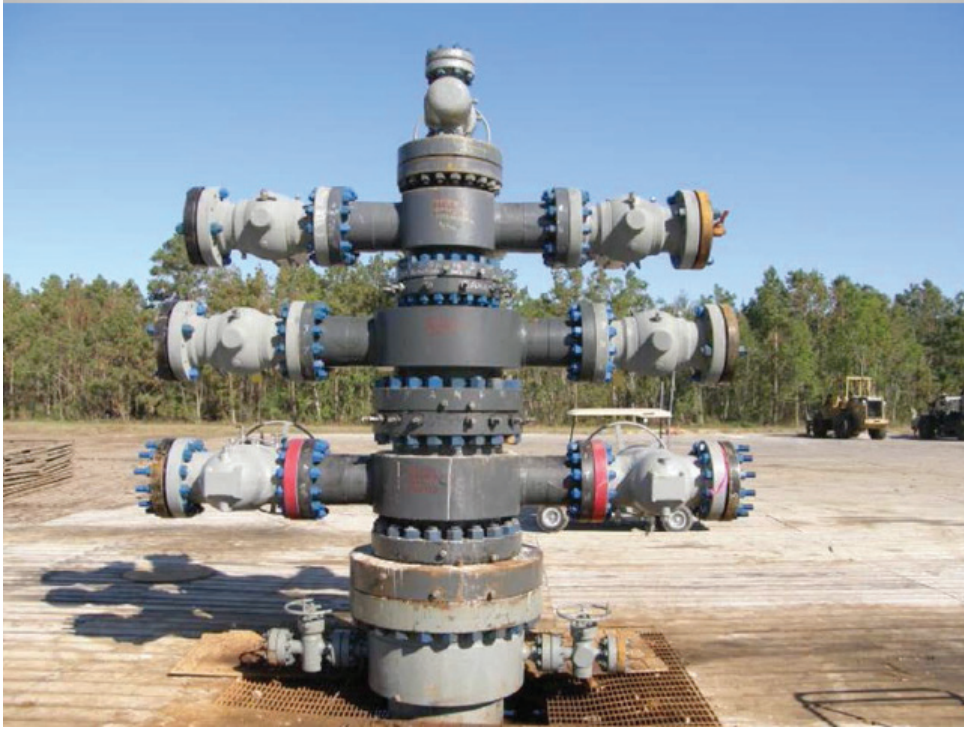
Figure 10-4: Example Salt Cavern Well Wellhead Configuration During Gas Storage Operations
