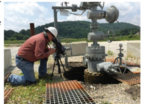
Figure 6-3: Surveying Wellheads for Potential Fugitive Emissions Source: ALL Consulting, 2015
