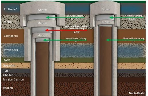
Note: Horizontal/lateral section is not included in this illustration \*Lowest Underground Source of Drinking Water (USDW) EERC LJ57056.
