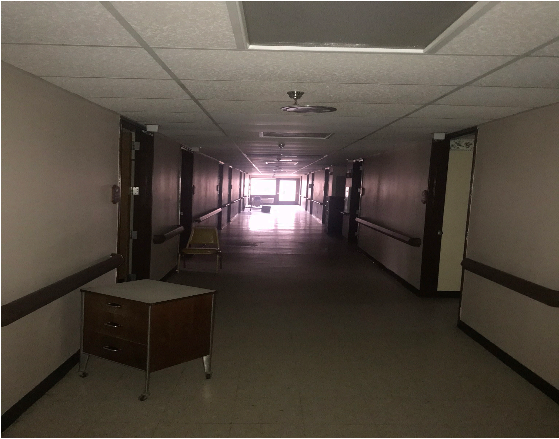
- Bldg 1 Hallway (Nursing Home) - ACM sheet flooring beneath floor tiles throughout bldg. 1-3 - ACM - Texture & Joint Compounds of the wall systems throughout the bldg 1-3
