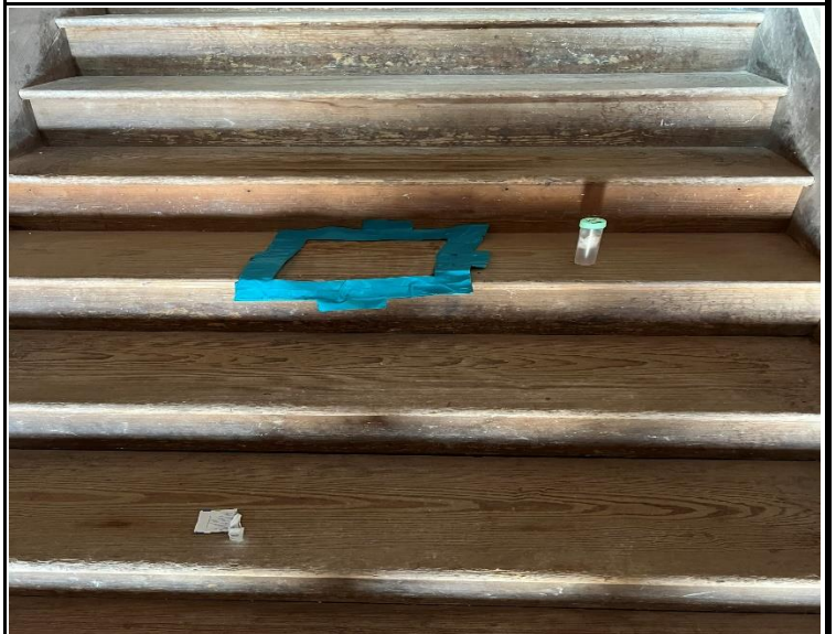
Photo 28: Thomas Apartments LBP Abatement Clearance Sampling Staircase
