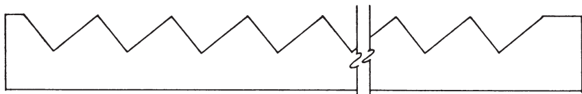
STRINGER LAID OUT
